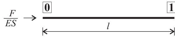
Figure A.1: A free-free beam subject to longitudinal excitation in the end 0
