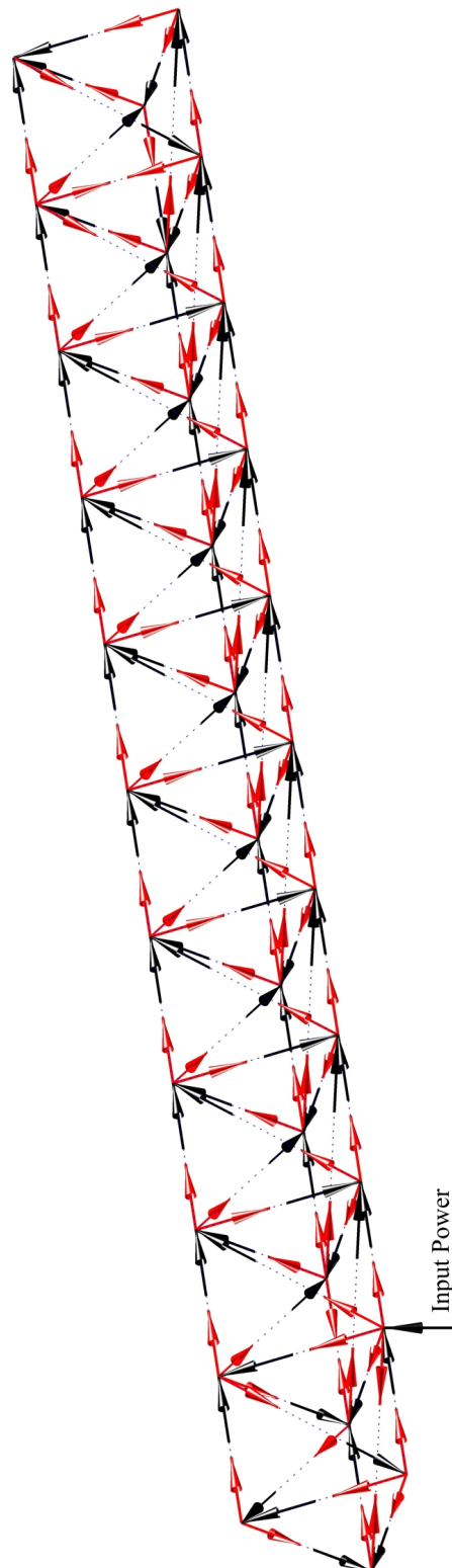
Figure 3.24: Diagram showing the direction of power flow in the structure. Results are for the sum of power flow over the frequency range 20 Hz - 1kHz.
