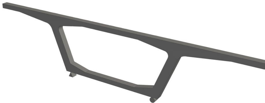
Figure 8.19 – One-Foot Section of Typical Cross Section
