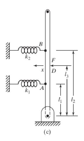
If the force F is applied at another point D of the rigid bar as shown in the figure, the equivalent spring constant referred to point D can be found as
