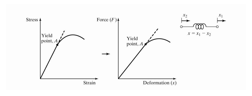
Often springs are nonlinear. The behavior shown in the figure (force as a function of the deformation) exhibits nonlinear behavior after point A.
