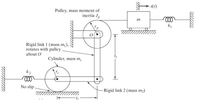
$$T = \frac{1}{2} m \dot{x}^2 + \frac{1}{2} J_p \left(\frac{\dot{x}}{r_p}\right)^2 + \frac{1}{2} \left(\frac{m_1 l_1^2}{3}\right) \left(\frac{\dot{x}}{r_p}\right)^2 + \frac{1}{2} m_2 \left(\frac{\dot{x} l_1}{r_p}\right)^2$$
