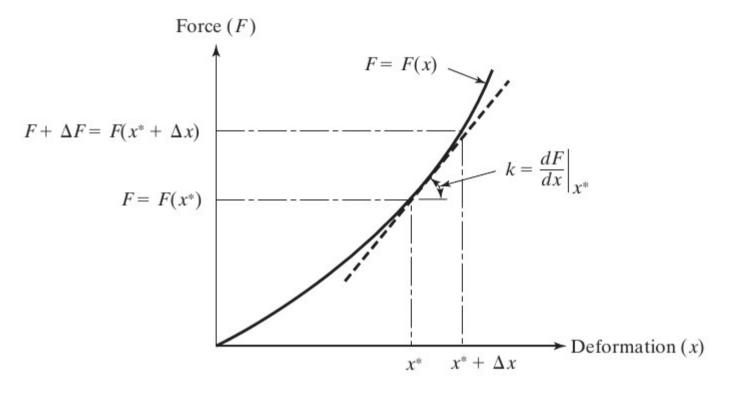
For small displacements around an equilibrium point, the first derivative is usually enough to represent the stiffness
