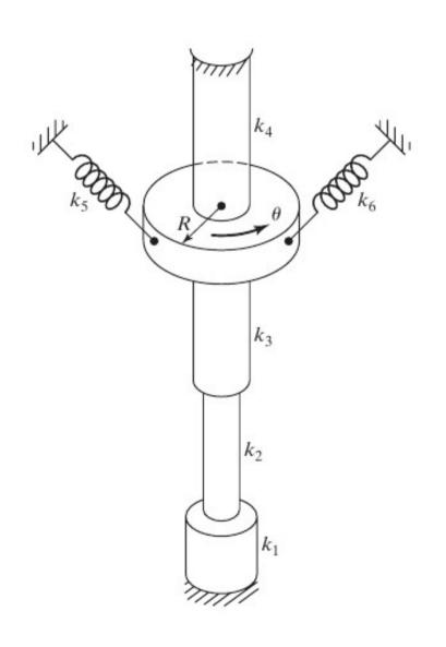
Determine the equivalent spring constant of the system shown in the figure
