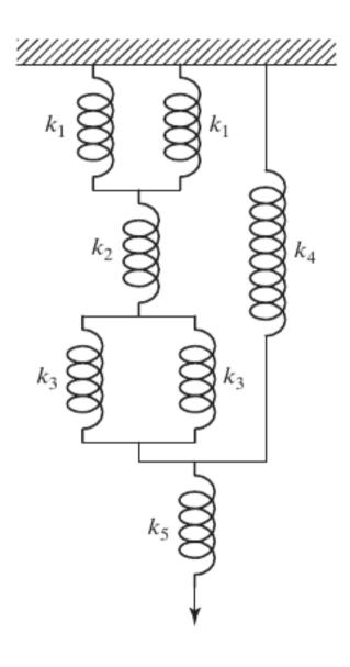
Determine the equivalent spring constant of the system shown in figure
