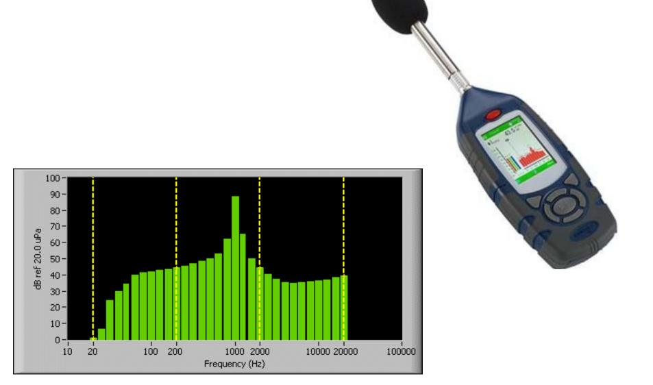
**Decibel**. The various quantities encountered in the field of vibration and sound (such as displacement, velocity, acceleration, pressure, and power) are often represented using the notation of decibel. A decibel (dB) is originally defined as a ratio of electric powers:
