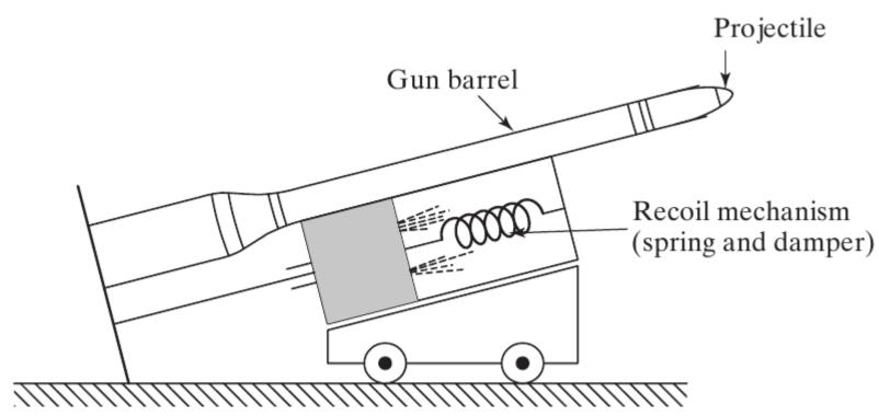
In a particular case, the gun barrel and the recoil mechanism have a mass of 500 kg with a recoil spring of stiffness 10,000 N/m. The gun recoils 0.4 m upon firing.
