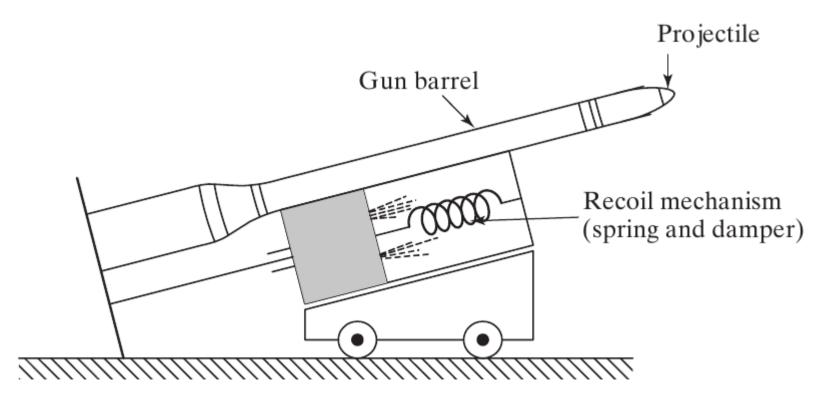
Since it is desirable to bring the gun barrel to rest in the shortest time without oscillation, it is made to translate backward against a critically damped spring-damper system called the recoil mechanism.
