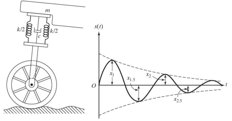
Find the necessary stiffness and damping constants of the shock absorber if the damped period of vibration is to be 2s and the amplitude x1 is to be reduced to onefourth in one half cycle (i.e.,  $X_{15} = X_{1/4}$ ). Also find the minimum initial velocity that leads to a maximum displacement of 250 mm.
