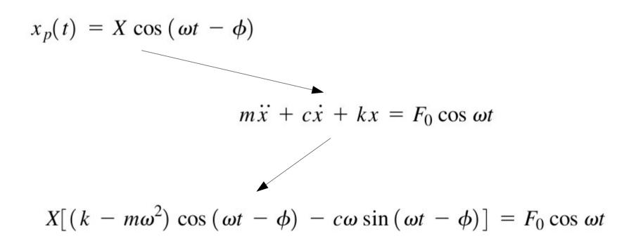
$$X[(k - m\omega^2)\cos(\omega t - \phi) - c\omega\sin(\omega t - \phi)] = F_0\cos\omega t$$
