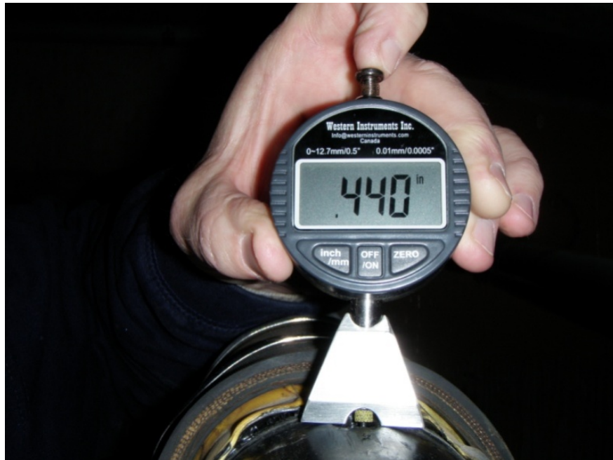
Figure 53. Photo. Dial gauge used to determine the depth of a grout air void.
