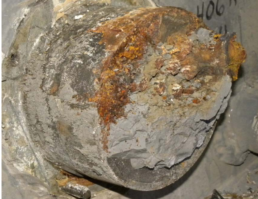
Figure 32. Photo. Opened tendon end revealing type 4 grout (bottom half), type 1 grout (center region), and strand corrosion products (upper region).
