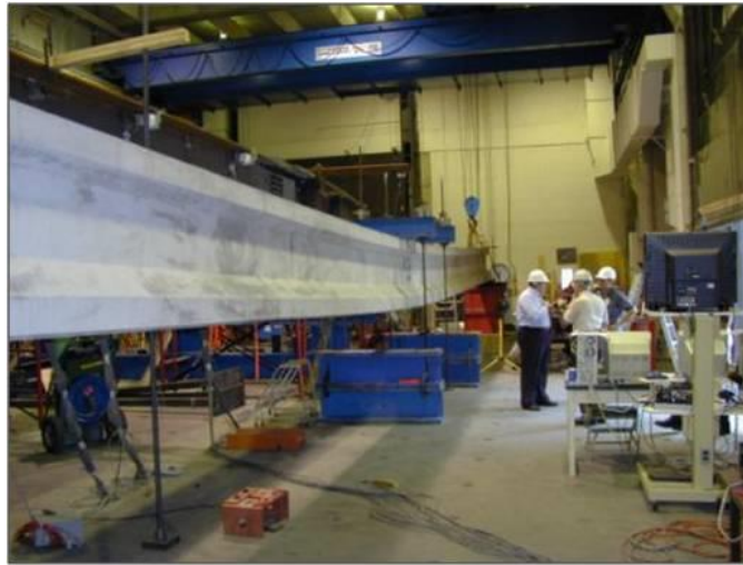
Figure 10. Photo. Flexural test of an AASHTO Type II girder made of UHPC
