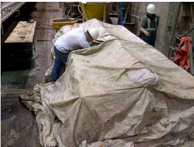
Figure 3. Typical curing chamber used at each plant for the NRCC test program
