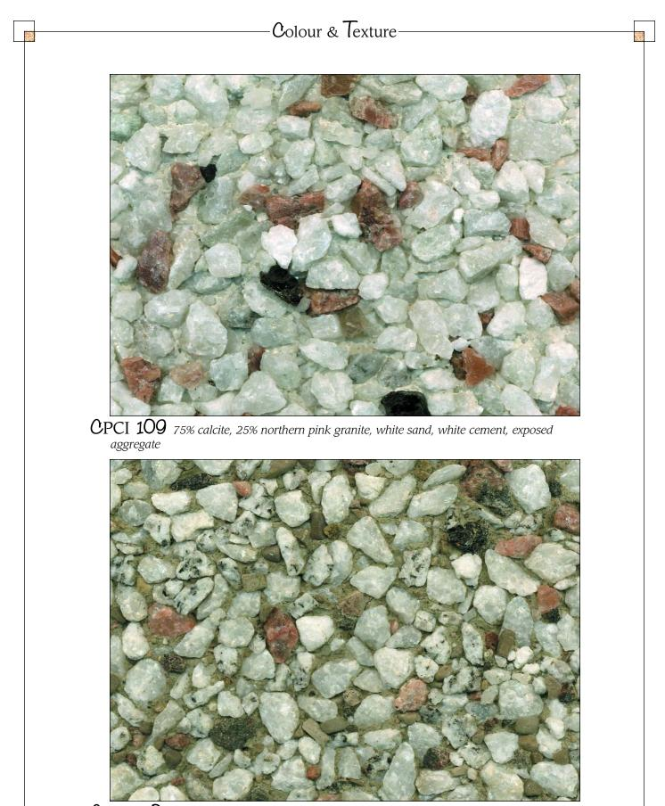
**CPCI 110** calcite, light grey granite, empire red granite, northern pink granite, concrete sand, grey cement, exposed aggregate
