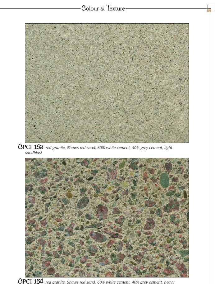
CPCI 164 red granite, Shaws red sand, 60% white cement, 40% grey cement, heavy sandblast
