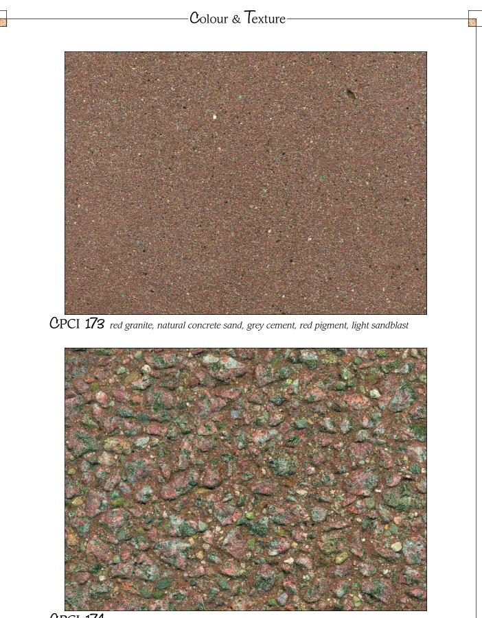
CPCI 174 red granite, natural concrete sand, grey cement, red pigment, heavy sandblast
