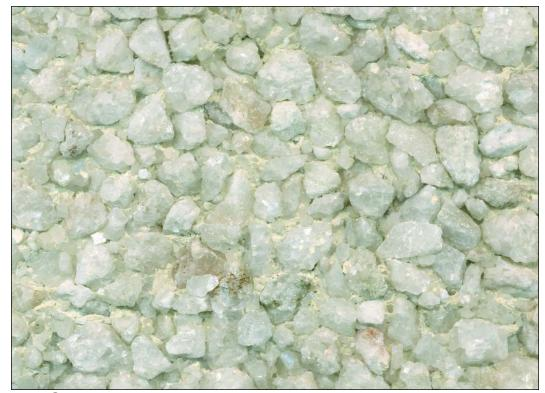
CPCI 104 calcite, white sand, white cement, exposed aggregate
