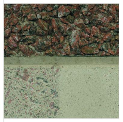
darker in colour the sample becomes darker. With even deeper sandblasting (or an exposed/washed finish), the coarse aggregates are now being exposed and little of the matrix is visible. The sample now shows the true colours of the fine and coarse aggregates in the concrete mix. Feel free to mix and match, but it is best to stay with the same concrete mix throughout.
