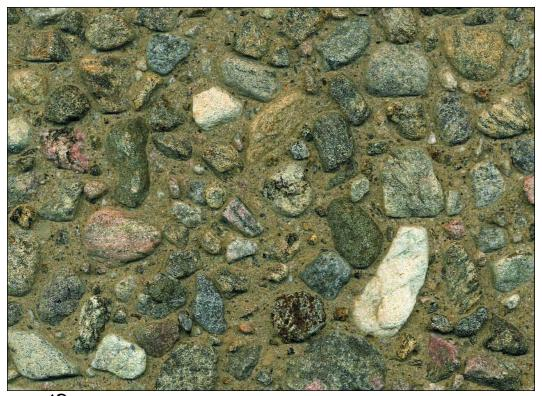
CPCI 140 <sup>3</sup>/<sub>8</sub>-<sup>5</sup>/<sub>8</sub> inch multicoloured river gravel, natural brown sand, grey cement, dark yellow pigment, medium sandblast
