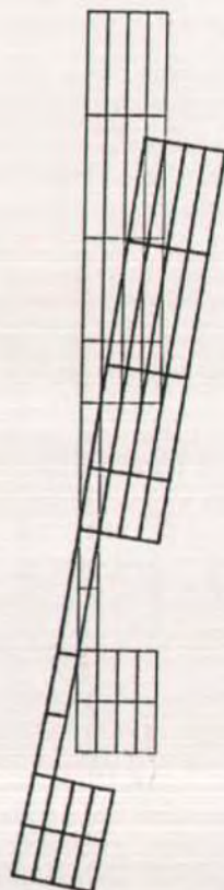
Fig. 10. Midspan deflection of pocket spandrel (superimposed dead load plus live load).
