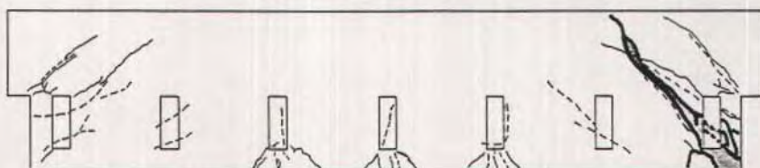
(B) FRONT ELEVATION OF SPECIMEN 3-(PHASE 1) AT ULTIMATE LOAD
